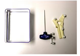
Fig. 4 Phantom box, tracked needle, and registration device
